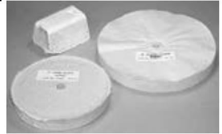
**White compound (aluminum oxide)** requires friction heat on cloth wheel for transfer. #10688.....\$6.50
