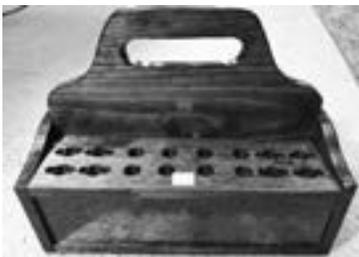
**Classroom toolbox (no drawer)** made from 1/2" pine, stained and sealed. Weight is 3 lbs. without tools.
